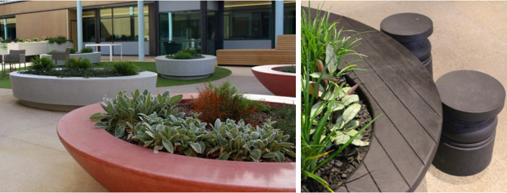
Prefabricated planters to be planted with seasonal planting for year around activities, timber slats on edges for seating. Typical seating height 450-500mm above FFL.
